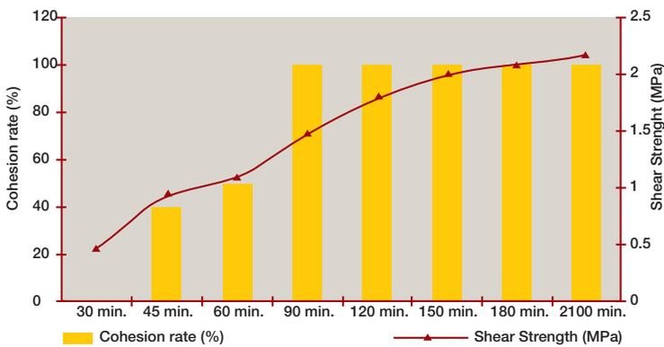
Curing time of 25-30 minutes at room temperature allows the assembled parts to be handled
