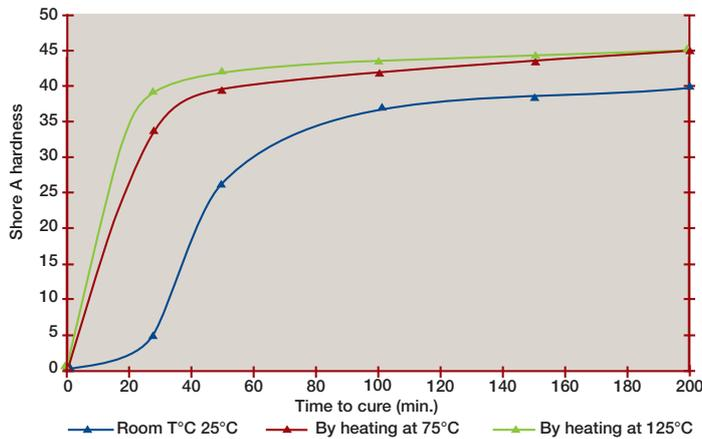
Complete curing in confined environment in high section thickness
